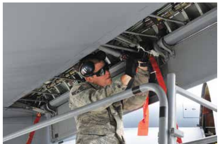
Senior Airmen Justin Keck installs leading-edge flap locks on a KC-135 Stratotanker during annual training in Alpena, Mich.
